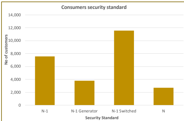
Figure 10: Customer substation security ranking (Source: Eastland analysis)
