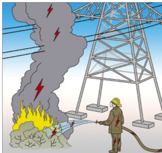
Figure 15: Electric current can arc through smoke and flames, as well as travel through water jets.
